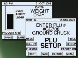
Large 320 x 240 resolution, backlit, blue LCD graphics display and 14 soft keys
